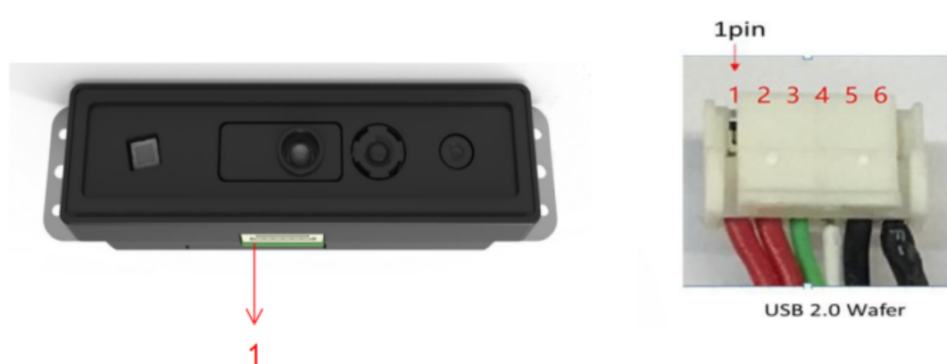
USB 2.0 Wafer interface definition (with PIN 1 position mark)
